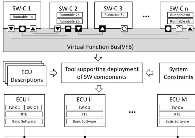
Fig. 1. AUTOSAR components, interfaces and runnables. (Adapted from [1])
