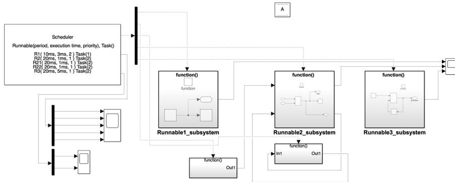
Fig. 11. Splitting a single runnable into three subsystems
